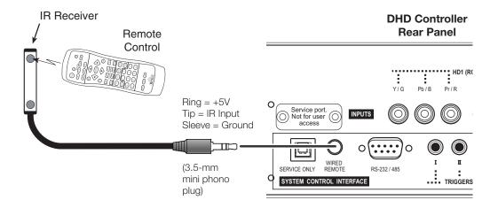
Figure 3-18. External IR Receiver Connection
